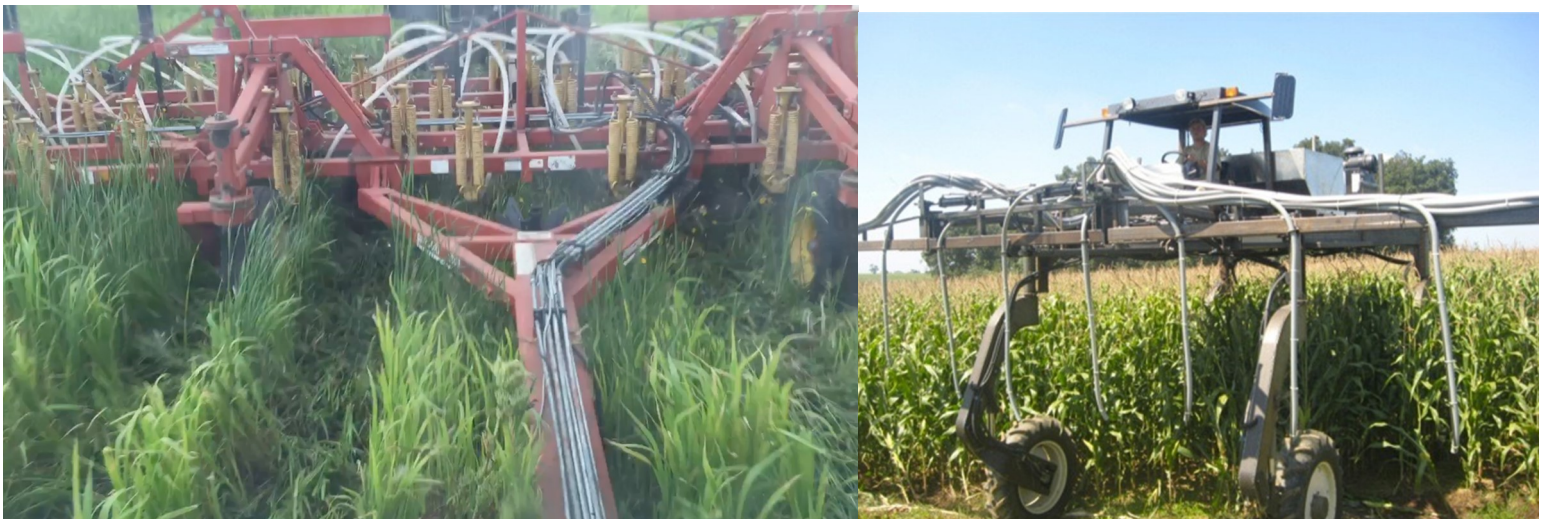
Examples of equipment to plant cover crops photos courtesy of Kevin Elmy, Friendly Acres Seed Farm. Photo above left: modifies sprayer. Photo above right: Herd Spreader. Photo below left: 1986 8800 Bourgault airseeder. Photo below right: modified “retired” detasseler.
